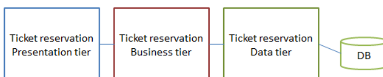
Figure 4.1: Software stack for ‘ticket reservation’ web application
